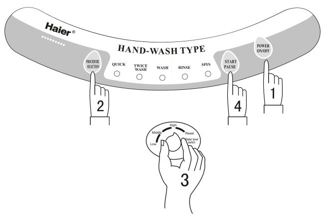
1 Push the "Power On/Off" button to switch on the power
